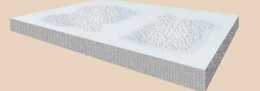
As anhydrite cures, a weak layer of laitance is formed on the surface.
