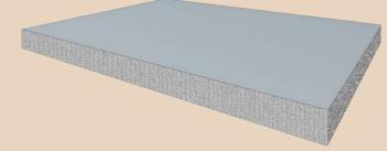
Anhydrite screeds are made from inert fillers such as sand, with a binder system based on calcium sulphate. Consequently they can look very similar to a sand/cement screed.
